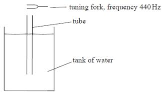
A tube that is open at both ends is placed vertically in a tank of water, until the top of the tube is just at the surface of the water. A tuning fork of frequency 440 Hz is sounded above the tube. The tube is slowly raised out of the water until the loudness of the sound reaches a maximum for the first time, due to the formation of a standing wave.
