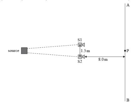
A person walking in a straight line from A to B observes that the intensity of sound alternates between high and low.
