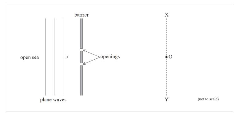
Plane water waves from the open sea are incident on the barrier and the openings act as point sources of waves. The distance from the openings to XOY is much greater than the wavelength of the wave. O is equidistant from the openings.
