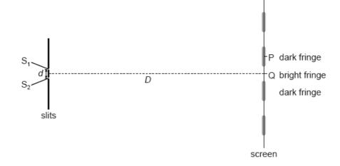
When red light of wavelength 660 nm is used the first fringe at P subtends an angle 0.0045 rad from midpoint of  $S_1$  and  $S_2$ .
